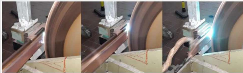
Burning arcs on the wheel: (left) good contact, (middle) arc elongation, (right) quenching
